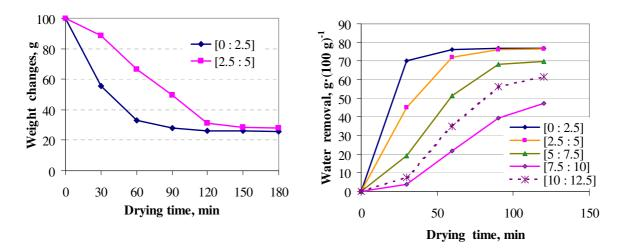
Fig. 4. Beer dregs layers weight changes during venting with temperature 35 °C
