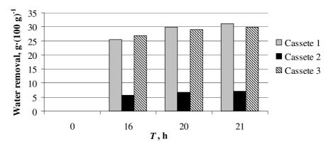
Fig. 3. Average moisture removal from 3 cassettes in 7.5 cm thick layer depending on the drying time *T*
