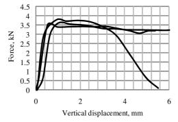
Fig. 1. Typical compressive load-displacement curves of hemp stem
